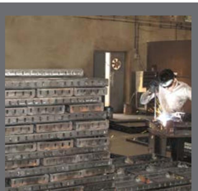
In addition to modular belt case (weld) there is another modular case or frame which is called bend case. This type of case is used in framing system to replace belt frame depending on customer's choice. The entire angles of this frame and its peripheral belts are bent by machines and a few number of its components are welded. It should be noted bend frame is not different from belt frame in terms of working procedure and using fittings and attachments.
