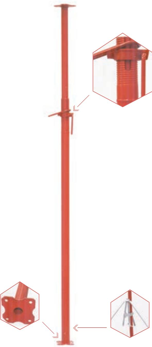
Prop made from two part that adjustable in length, up and down parts. The lower part is made of tube with a diameter of 60 mm and thickness is 2.5 mm. the upper part is made of tube with a diameter 50 mm and thickness is 2.5 mm too.
